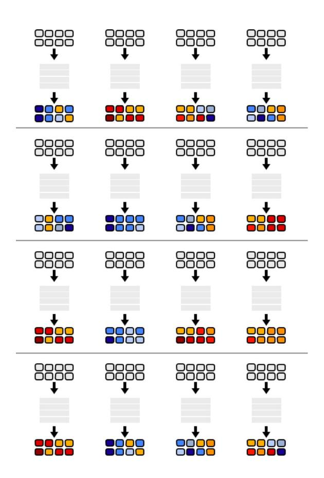
**16 cores x 8 ALUs/core = 128 ALUs 16 cores = 16 simultaneous instruction streams**
