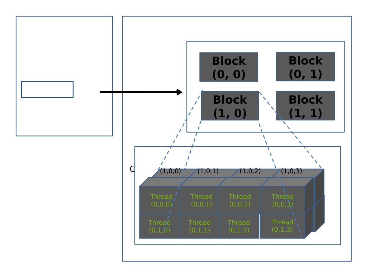
Note: Block index: (y, x), Thread index: (z, y, x)
